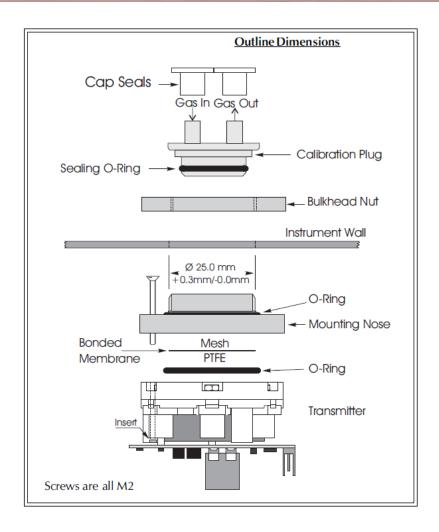
A diffusion mounting assembly, the 'nose' adaptor, has been designed for convenient mounting in a wide range of weatherproof housings. Moulded in resilient polyester, the nose adaptor requires a 25mm diameter hole in the outside wall of the housing to allow installation. A bonded membrane and mesh is employed to prevent the ingress of dirt and dust particles into the sensor.
