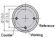
All dimensions are in millimeters. All tolerances are ±0.2mm.
