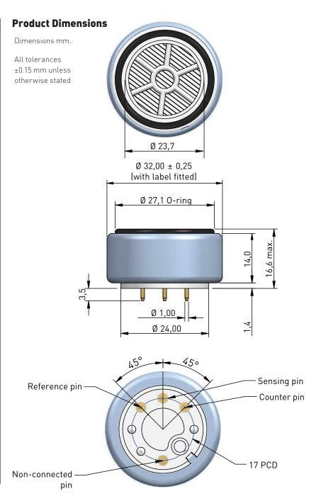
**Important Note:** Connection should be made via recommended mating parts only. Soldering to the sensor will damage it and invalidate the warranty.
